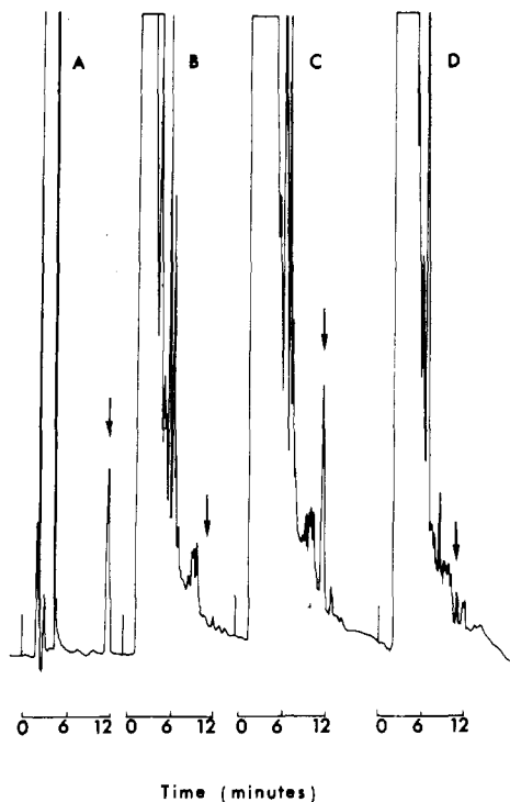
Figure 4. HPLC chromatograms of potatoes: (A) pencycuron standard, 10 ng (equivalent to 0.08 ppm); (B) untreated control soil; (C) control potato fortified with 0.08 ppm of pencycuron (100% recovery); (D) control potato fortified with 0.01 ppm of pencycuron (85% recovery).
